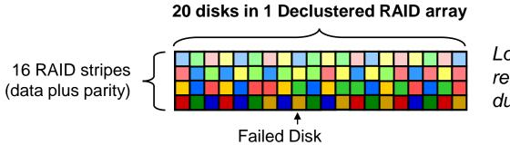
Load on files accesses are reduced by 4.8x (=19/4) during array rebuild.
