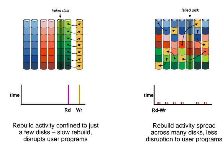
Rebuild overhead reduced by 3.5x
