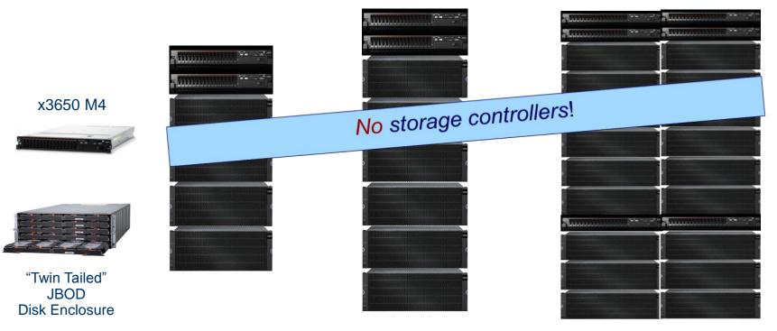
Model 24: Light and Fast 4 Enclosures, 20U 232 NL-SAS, 6 SSD 10 GB/Sec Model 26: HPC Workhorse! 6 Enclosures, 28U 348 NL-SAS, 6 SSD 12 GB/sec High-Density HPC Option 18 Enclosures 2 - 42U Standard Racks 1044 NL-SAS 18 SSD 36 GB/sec
