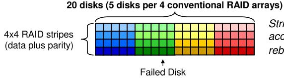
Striping across all arrays, all file accesses are throttled by array 2's rebuild overhead.
