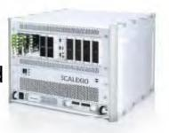
HiL simulation provides an effective platform by adding the complexity of the plant under control to the test platform. The complexity of the plant under control is included in test and development by adding a mathematical representation of all related dynamic systems.
