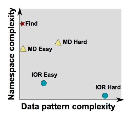
IOR Easy: This is what is used during the procurements, where we measure the most efficient I/O pattern, user can declared the parameters and we save one file per MPI process
